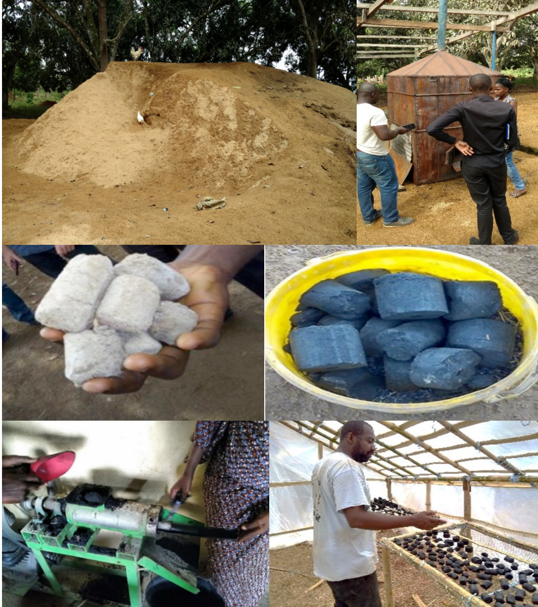
Figure 2.3. Rice Husk Briquettes. Left top: pile of rice husk behind the rice mill; Right top: rice husk carbonizer; Left middle: original dried husk biomass briquette without carbonization (pyrolysis); Right middle: briquettes using carbonized rice husk (these burn cleaner and produce more energy per unit of mass); Left bottom: motorized briquette press; Right bottom: drying of briquettes in a greenhouse.
