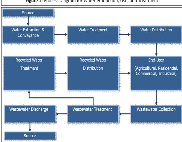
Figure 1: Process Diagram for Water Production, Use, and Treatment
